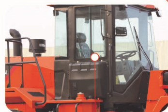
Emergency escaping window
